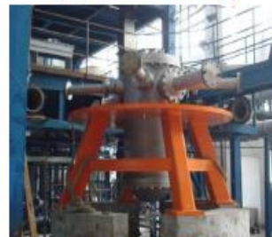
Hydraulic and FIV test ( NPIC )
