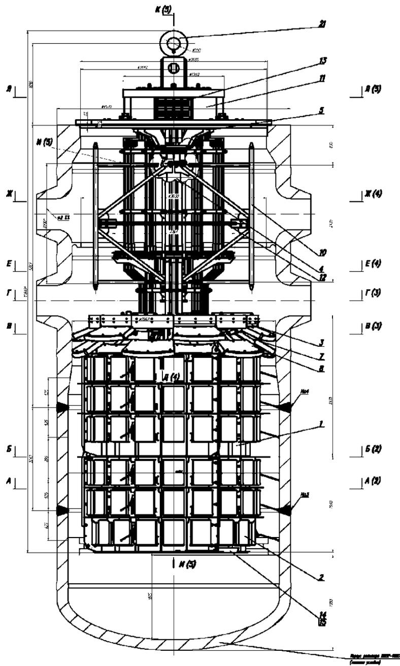
Heating device in reactor vessel
