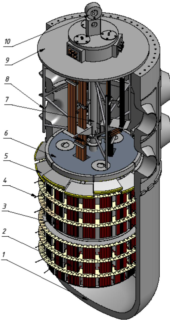
**2)** Heating device contains a lid of biological protection and two heater units connected with a bar with membrane installed on it linked with a curtain and a draw bar.
