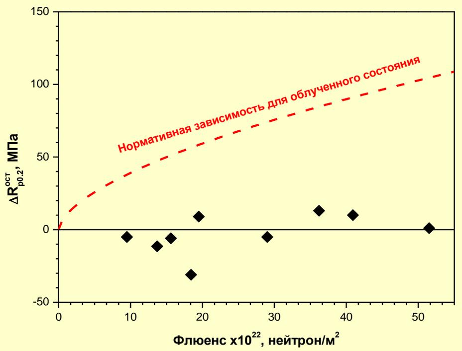
Possibility for almost total recovery of material structure and properties in VVER reactor vessel as a result of recovery annealing after irradiation within the range of neutron fluence corresponding to the design one as well as to prolonged up to 60 years operation period was proved experimentally. This demonstrates possibility of recovery annealing application to provide operation of reactor vessels up to 60 years and more.
