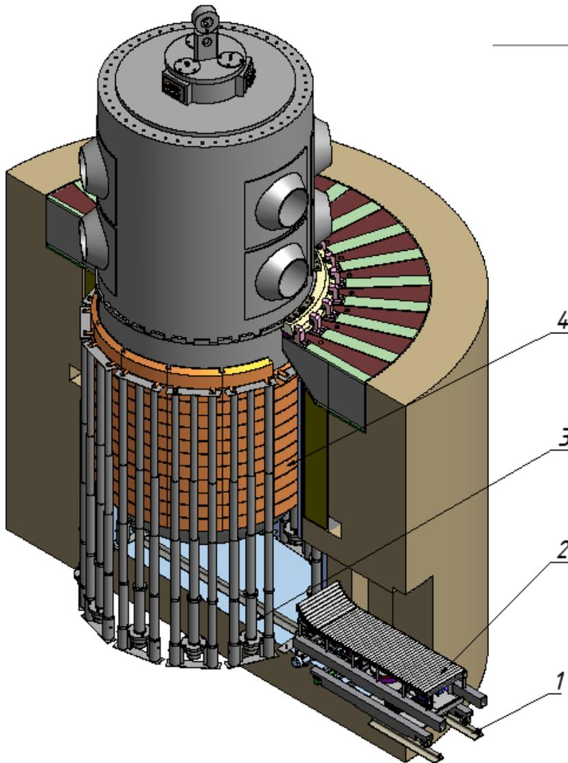
*Thirteen vertical «straps» of heat insulation (metal box filled with heat insulation material).*
