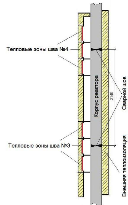
***The scheme of double-side heating (heating of internal and external surface of vessel)***
